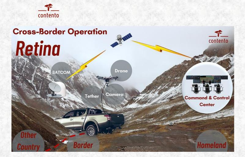
Cross-border operations do not have a fixed surveillance infrastructure. That's why Retina is designed for use beyond borders. With its tethered structure, the drone can be raised up to 100 meter height, stays in the air for an unlimited time, and the surveillance beyond the border is never interrupted. In addition, data that cannot be jammed thanks to its tethered structure can be transferred to the command & control center via SATCOM if desired.
